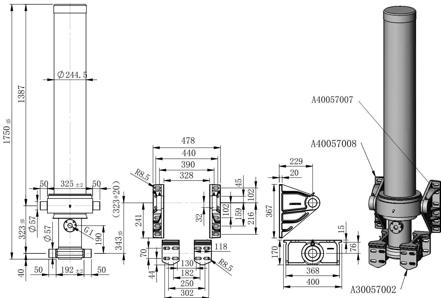
mounting dimension 323 mm + 20 mm min pull out
